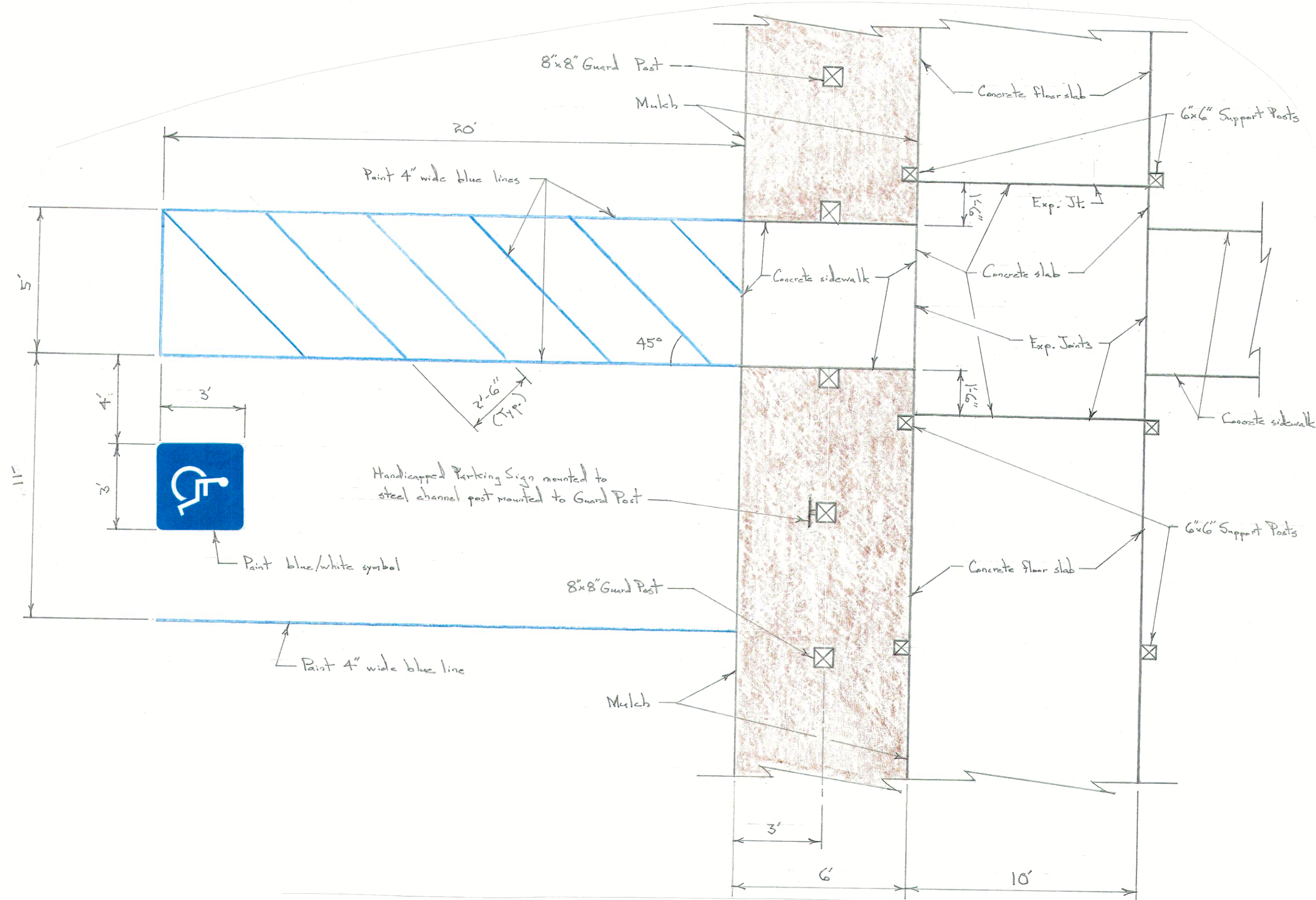
HANDICAPPED PARKING AREA DETAIL
